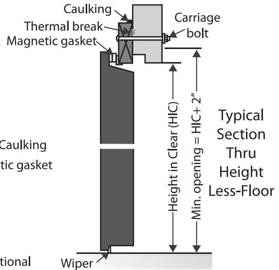
Typical Section Thru Height Less-Floor
