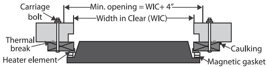
Typical Section Thru Width
