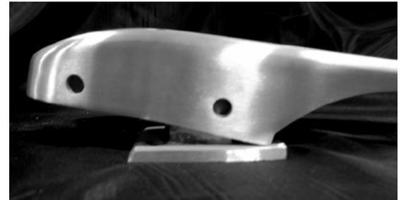
4. Holding handle down securely, inset handle pin through hole of handle and base. Push or use hammer to tap pin lightly through holes until groove of pin is lined up with center slot of base.
