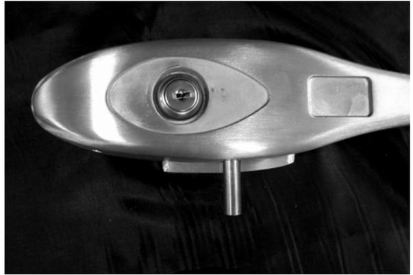
5. Insert clip through slot of base on to groove of pin using needle nose pliers.
