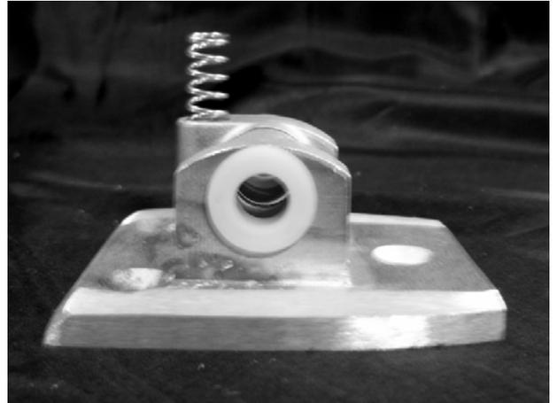
3. Place handle over base, lining up side holes of handle with side holes of base. Note: Handle will resist due to spring tension as it's forced down. Make sure opposite end of spring has engaged handle boss.
