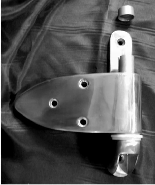
2. Turn hinge upside down with back of hinge facing you. Rest base on protected surface. Using rubber tipped hammer forcefully strike side of hinge blade close to the base.
