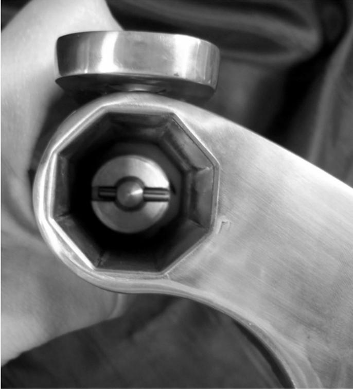
6. Rest base on protected surface. Using rubber tipped hammer forcefully strike side of hinge blade close to the base. Repeat as necessary until hinge blade is resting fully on nylon hinge.
